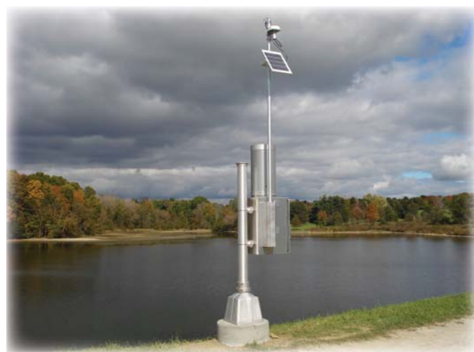
A StormLink Monitoring Station was installed at Chippewa Dam III-A – Hubbard Valley by MWCD Staff. Information on rainfall and flood pool stage is gathered continuously and can be accessed remotely.
