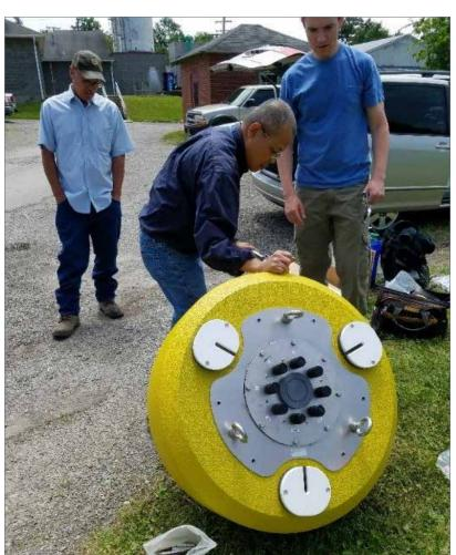
The data sonde, installed in Tappan Lake at the Cadiz water supply intake, will provide continuous data collection of water quality parameters.
