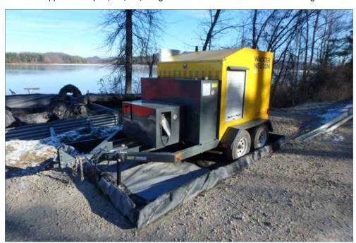
Individual water withdrawal pump during cold weather operations.
