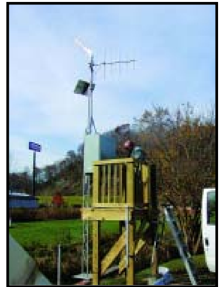
The early flood warning system at Duck Creek will consist of Installation of five combined stream and rain gages (similar to the one shown in the above photo) and two stand alone rain gages. Once completed, the system will also include a computer monitoring station for each county, transmitters, gage equipment enclosures and security fencing.
