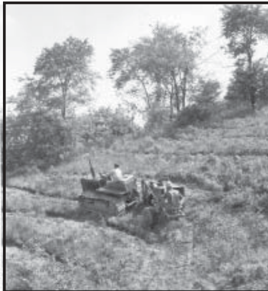
Steep slopes and abrupt turns over rough land are no handicap to this unusual “new” hydraulic control tree planter, developed by H.P. Garritt, Soil Conservation Service forester with the MWCD.
